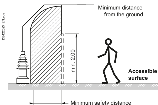
Fig. B14 Protection by installation of barriers. The safety distances are fixed by IEC 61936
