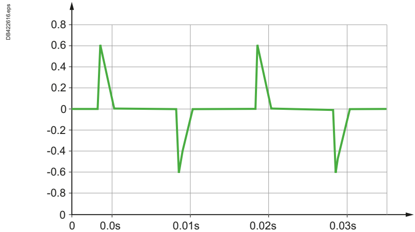
Fig. M7 Typical current waveform of a compact fluorescent lamp
